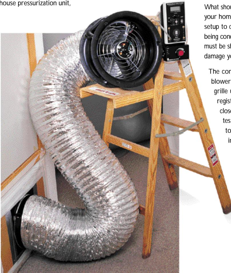
a high-powered fan set up in a doorway and connected to pressure gauges, to pressurize first the entire house and then the house with the duct system blocked off. This method is less accurate than the duct tester method and is not used as often.
