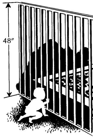
Guidelines recommend eliminating handholds and footholds and minimizing the size of openings in a barrier's construction.
